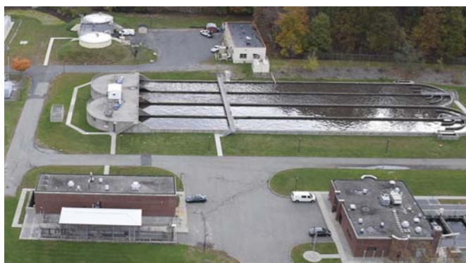
Figure 3. Oxidation ditch configuration for modeling.
